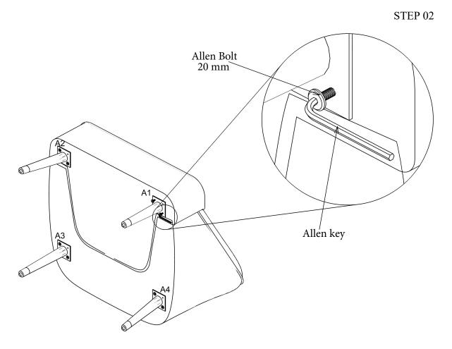
Fix the Part-A & Part-B with using Allen bolt M8x20 mm with help of Allen key at position A1,A2,A3&A4 as shown in Fig.
